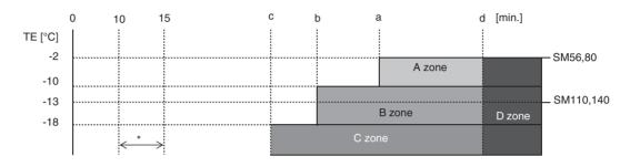
\* From 10 minutes to 15 minutes after a heating operation started, the minimum value of TE is stored in memory as TEO and the minimum temperature of TO as ToO.
