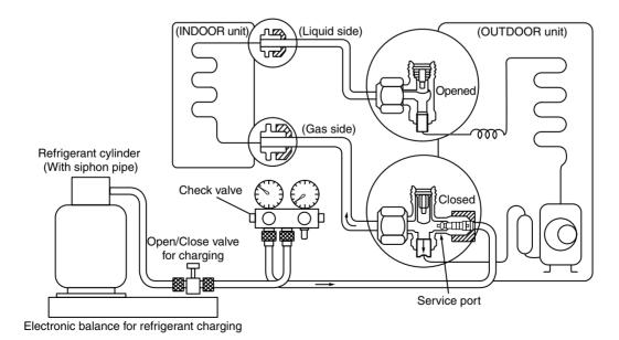
Fig. 6-4-1 Configuration of refrigerant charging
