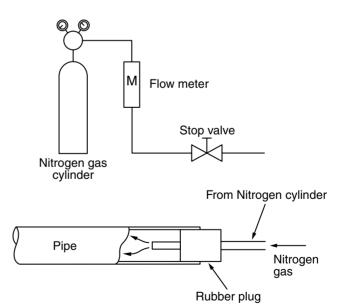
Fig. 6-5-1 Prevention of oxidation during brazing
