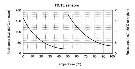
\* As TH sensor (Outdoor unit heat sink temp. sensor) is incorporated in the outdoor control P.C. board, the resistance value cannot be measured.
