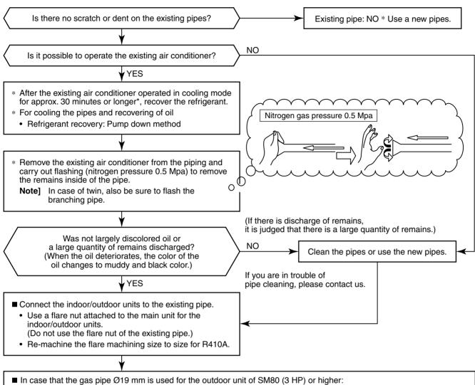
■ In case that the gas pipe Ø19 mm is used for the outdoor unit of SM80 (3 HP) or higher: (Gas pipe size of our R410A model 3 is Ø15.9 mm)
