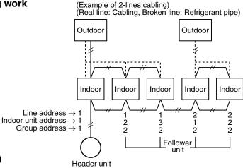
For the above example, perform setting by connecting singly the wired remote controller without remote controller inter-unit cable.
