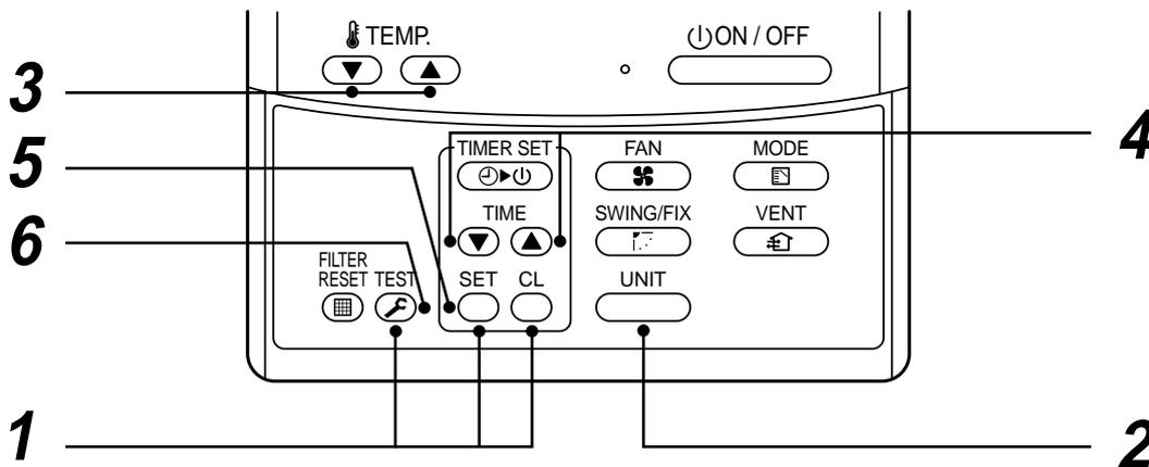
**1** Push **SET**, **CL**, and **TEST** buttons simultaneously for 4 seconds or more.
