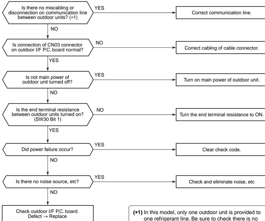
**(\*1)** In this model, only one outdoor unit is provided to one refrigerant line. Be sure to check there is no communication connection with outdoor unit in the other refrigerant line.
