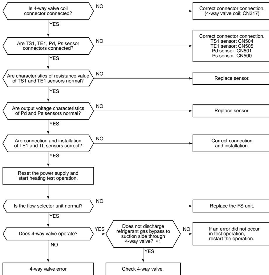
\*1 Check TS and TE temperature of the outdoor unit which compressors is operated.
