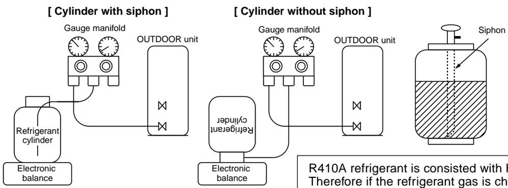
R410A refrigerant is consisted with HFC mixed refrigerant. Therefore if the refrigerant gas is charged, the composition of the charged refrigerant changes and characteristics of the equipment changes.
