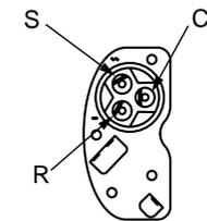
Details of compressor power connecting section
