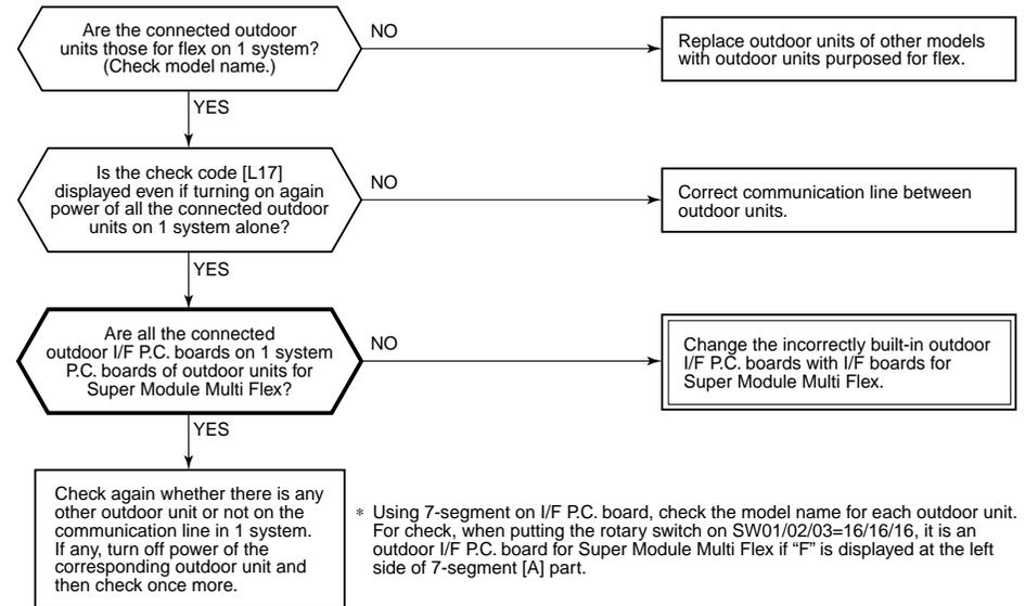
\* Using 7-segment on I/F P.C. board, check the model name for each outdoor unit. For check, when putting the rotary switch on SW01/02/03=16/16/16, it is an outdoor I/F P.C. board for Super Module Multi Flex if "F" is displayed at the left side of 7-segment [A] part.
