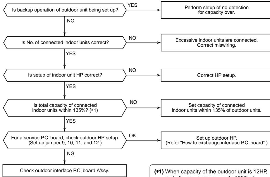
**(\*1)** When capacity of the outdoor unit is 12HP, up to the maximum capacity 120% of indoor units can be connected.
