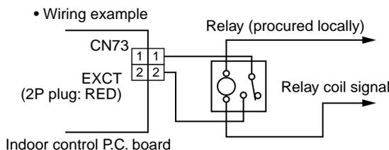
Note) Determine the cable length between the indoor or outdoor control P.C. board and the relay within 2m.
