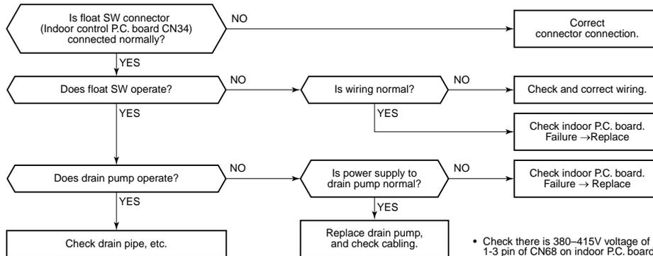
\* Check there is 380-415V voltage of 1-3 pin of CN68 on indoor P.C. board.
