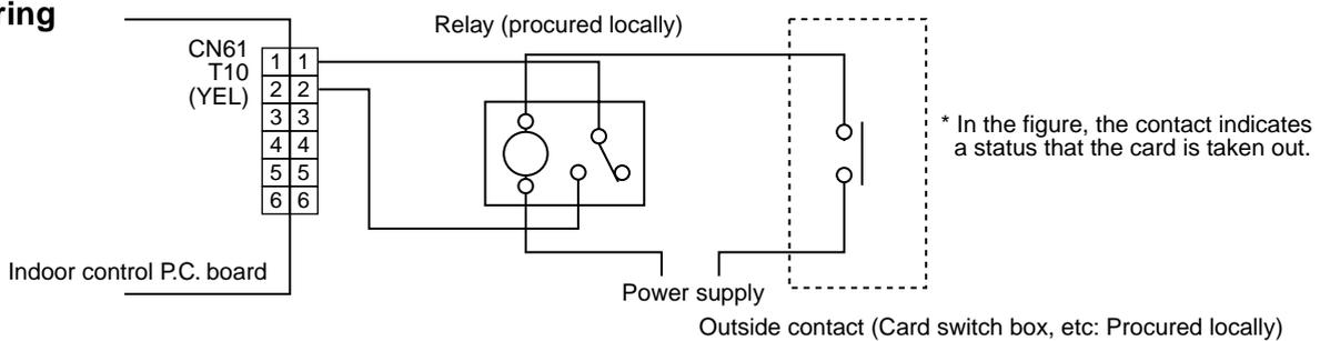
Note) Determine the cable length between the indoor control P.C. board and the relay within 2m.
