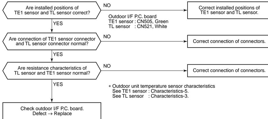
\* TE1 sensor : Outdoor heat exchanger temp sensor
